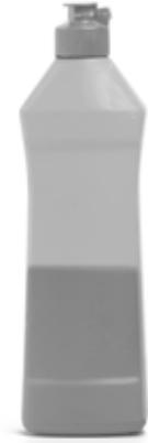
Examples of what a SWIR camera can capture: silicon, bruising inspection, fluids level inside opaque bottles.
